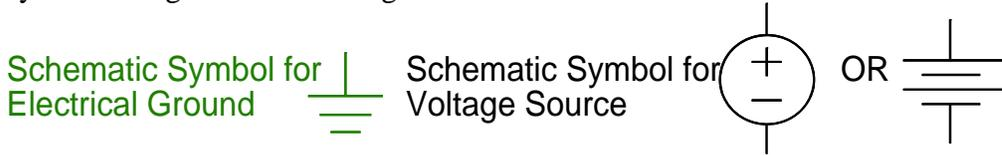
**Figure 5** Schematic Symbols: GND & Voltage Source
