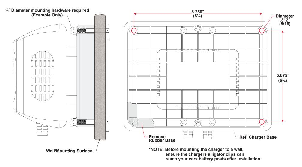
MOUNTING INSTRUCTIONS AND HOLE TEMPLATE FOR P/N 022-0221 CHARGER (Go to www.batterytender.com to download a full size hole template)
